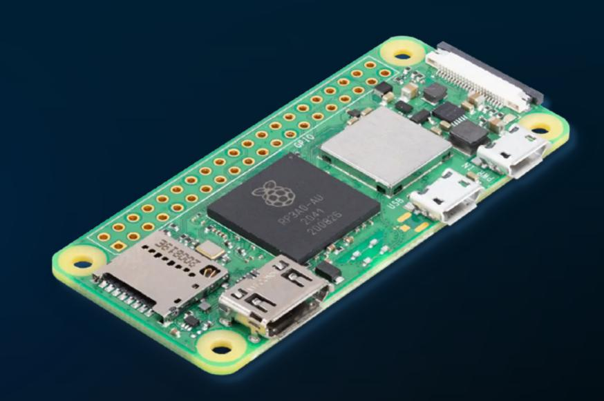
Pactus node on a Raspberry Pi Hardware: Raspberry Pi Zero
